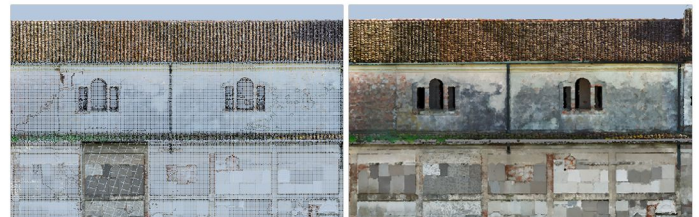
A 300 millions coloured point cloud and a high resolution densified solid image in CAD.
